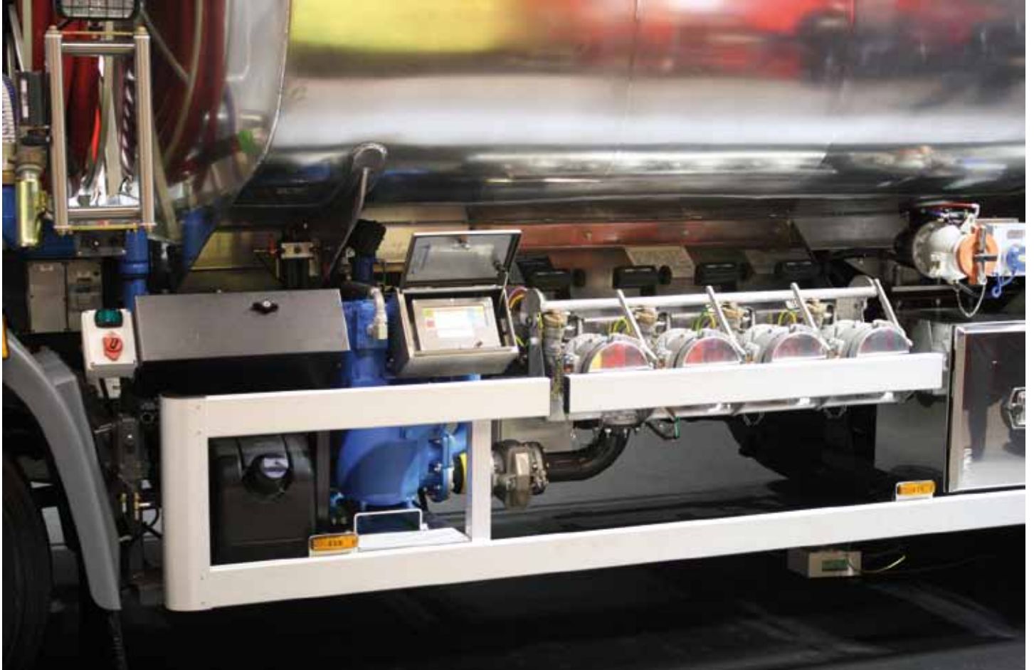
TCS Meters and Registers: suitable for service truck applications
